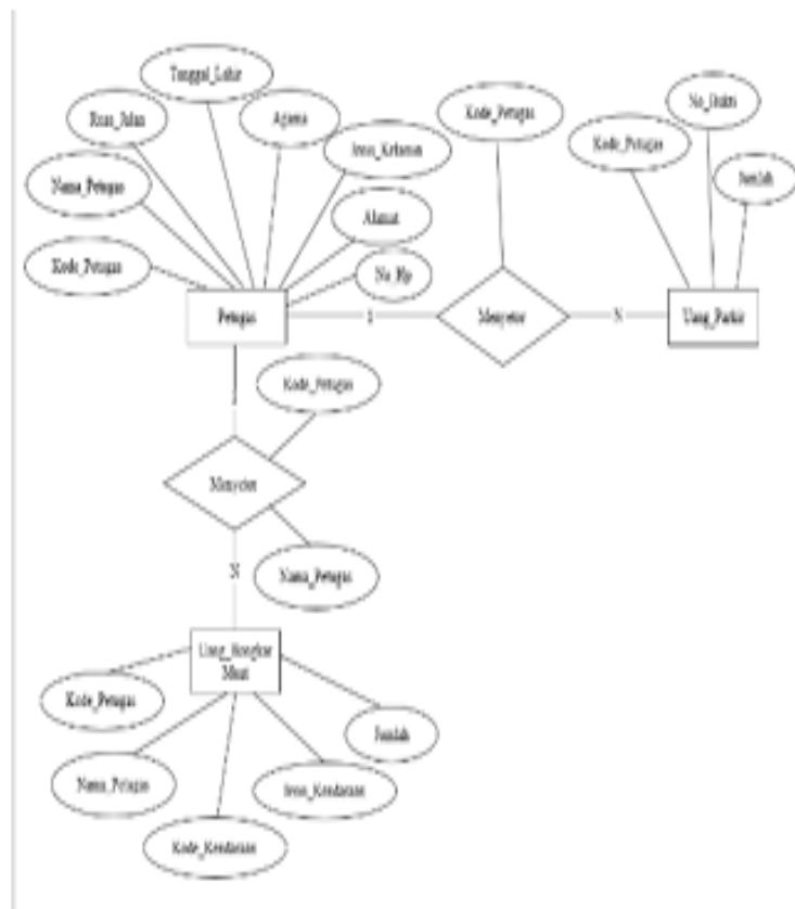
Figure 5. Entity Relationship Diagram (ERD) of the database design
